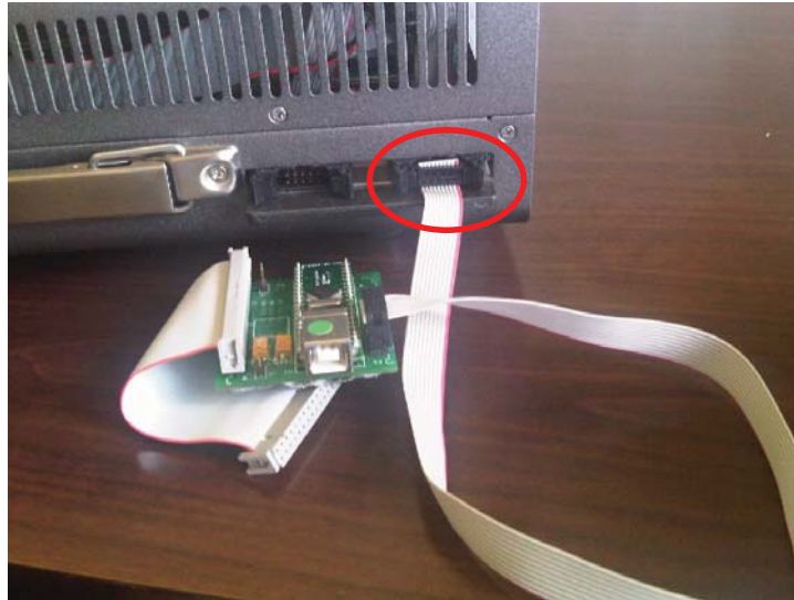
Figure 1 USB to SPI Adapter Board showing connection of SPI header [notice pin 1 (red) is on the right]
