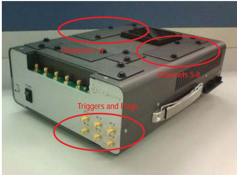
Figure 2 BTSD08 in a prototype enclosure showing High Speed Channel, Trigger and Flag locations
