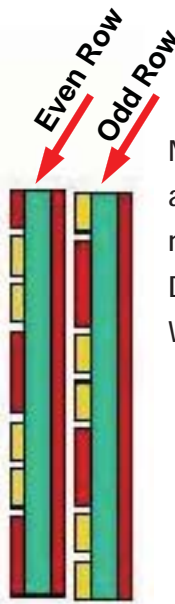
Figure 7-5: Even Differential Plug-in Module Wafer to Backplane Pin Mappings
